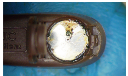
Figure 6: Battery fused in the battery compartment by rust/corrosion.
