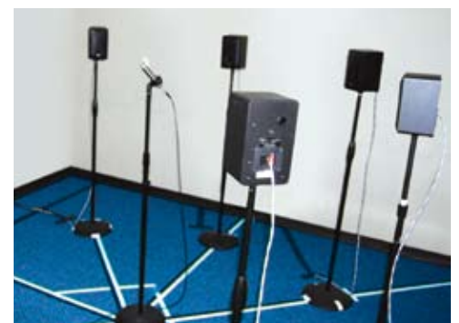
Figure 1: a) Schematic diagram of eight-loudspeaker array showing direction of noise sweep. b) Photo of eight-loudspeaker array with hearing aid under test located in the center.
